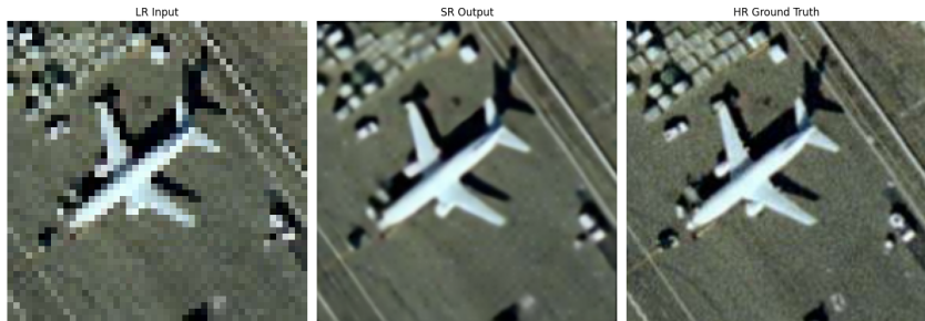
Figure 3: Example of qualitative analysis of DR-SCAN on \times 4 downsampled image from UCMerced dataset. From left to right: LR input, SR output using DR-SCAN, and HR ground truth.
