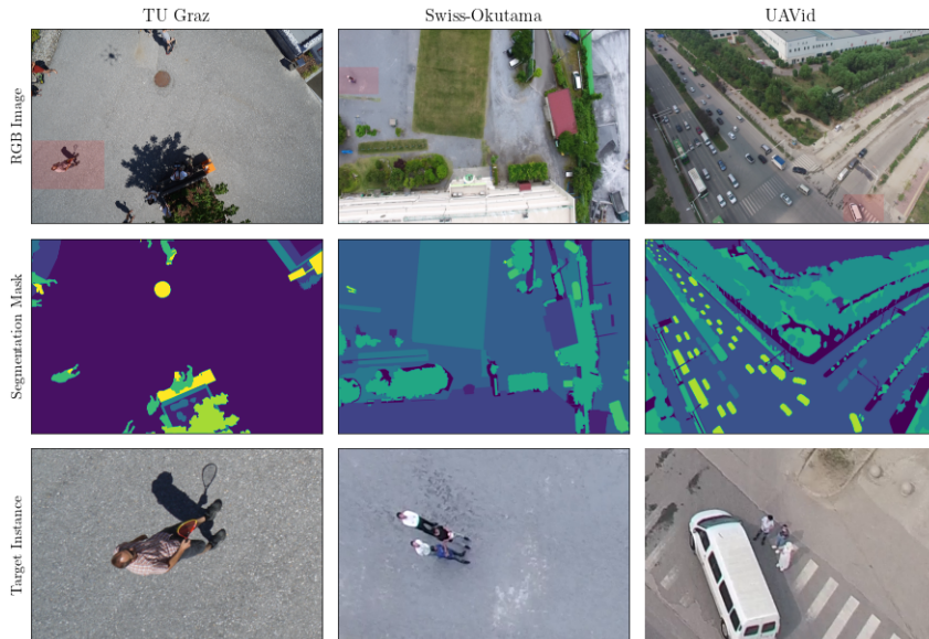
Figure 1: Example images from the TUGraz (left), Swiss-Okutama (middle), and UAVID (right) datasets, including the original RGB images (top row, red box denotes target instance), the corresponding segmentation masks (middle row), and a zoomed-in view of a target instance (bottom row).
